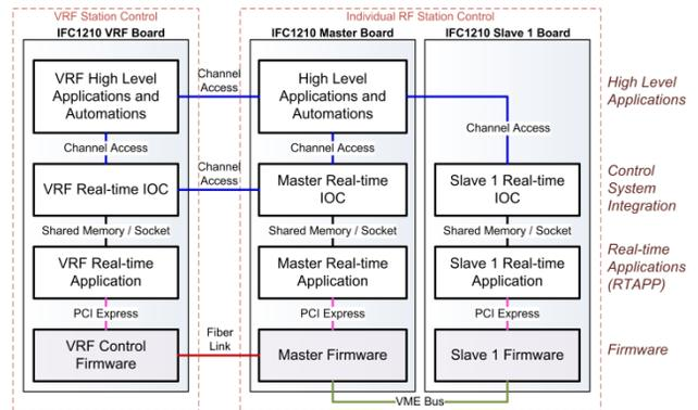
Figure 5: Architecture of LLRF firmware and software.
