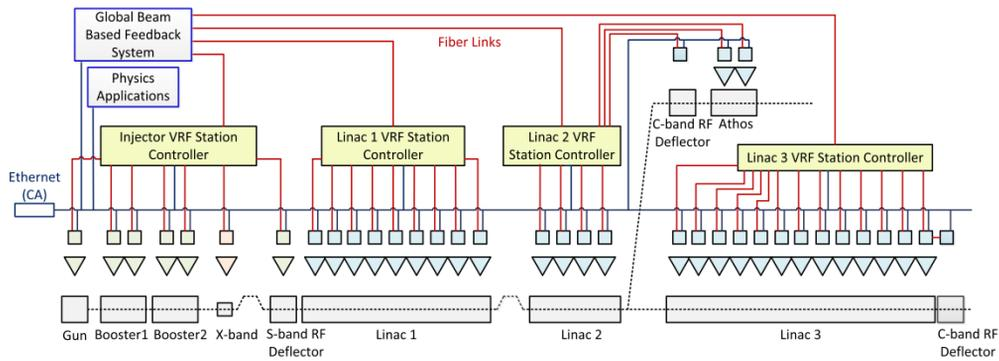
Figure 2: Virtual RF station controllers and LLRF networks.
