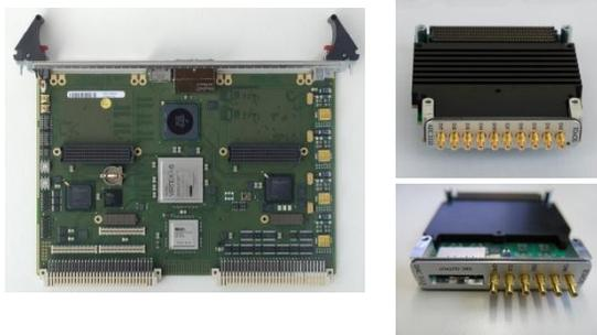
Figure 4: The IFC1210 (left), ADC3110 (right top) and DAC3113 (right bottom) boards.
