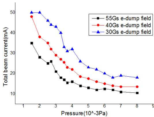
Figure 3: Total beam current of source VS operation pressure
