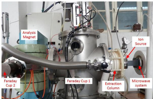
Figure 1: Ion Source Test Bench of PKU
