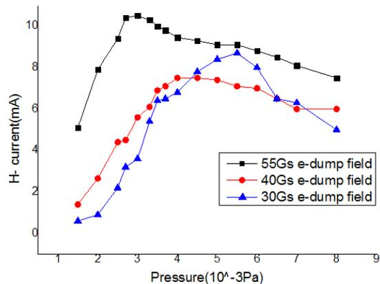
Figure 2: H<sup>-</sup> current VS operation pressure
