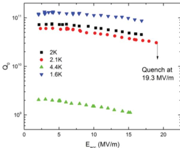
Figure 7: The  $Q_0$  vs  $E$  plot of 650 MHz cavity.
