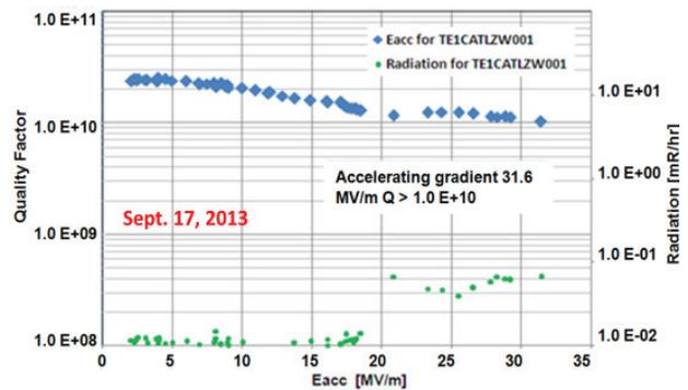
Figure 9: Test results of laser-welded single cell cavity.
