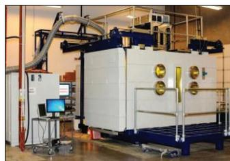
Figure 1: 15 kW electron beam welding machine.
