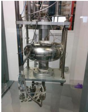
Figure 6: 650 MHz single-cell SCRF cavity.
