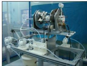
Figure 4: Electro-polishing setup.
