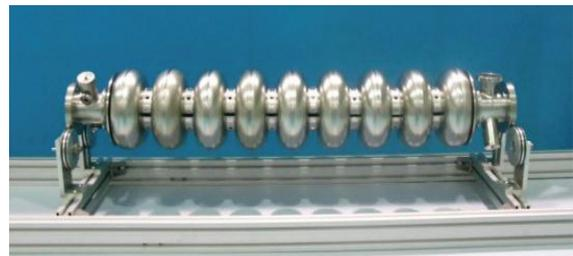
Figure 5: 1.3 GHz Nine cell SCRF cavity.
