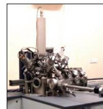
Figure 2: Secondary ion mass spectrometer.
