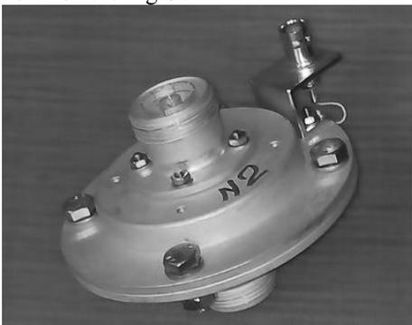
Figure 8: Solid state RF key.
