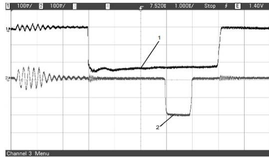
Figure 9: Pulse formed by RF key: 1 – envelope of incident RF signal, 2 – envelope of generated RF signal by RF key.
