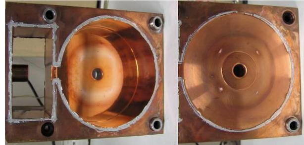
Figure 5: Internal cavity's surfaces.
