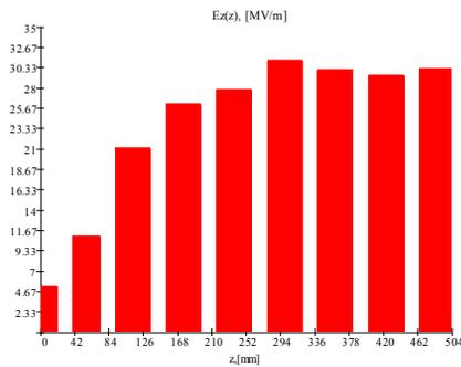
Figure 2: Histogram of the electric field amplitude with generator power of 2.5 MW.
