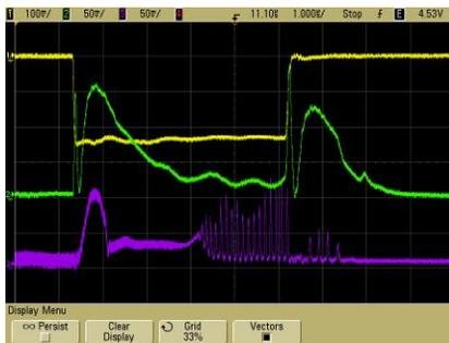
Figure 3: Oscilloscope of the multipactor effect: 1 (yellow) – input klystron's signal, 2 (green) – reflected from the structure signal, 3 (purple) – signal from the first accelerated cavity.
