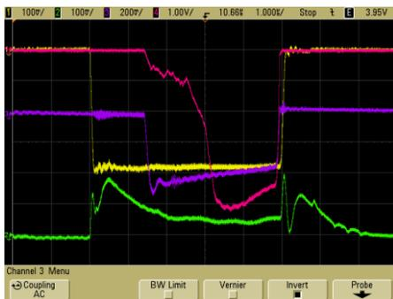
Figure 4: Oscilloscope of the envelope of the accelerated beam current: 1 (yellow) – input klystron's signal, 2 (green) – reflected from the structure signal, 3 (purple) – beam current from the electron gun, 4 (red) – accelerated beam current.
