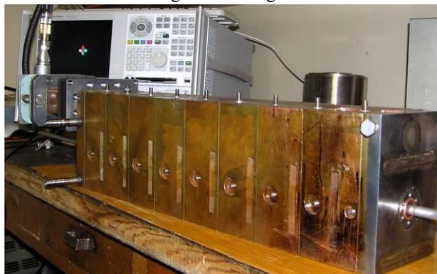
Figure 1: Accelerating structure with 9 accelerating cavities.
