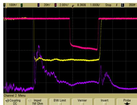
Figure 6: Beam current oscilloscope with amplitude of 120 mA and energy of 3.3 MeV: 1 (yellow) – input klystron's signal, 3 (purple) – reflected from the structure signal, 4 (red) – accelerated beam current.
