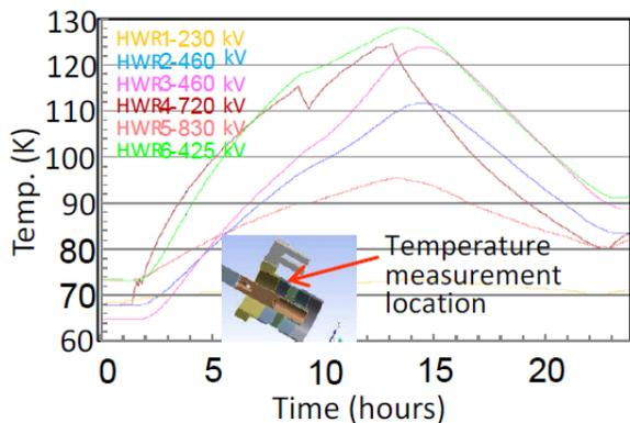
Figure 1: The couplers temperatures during operation of a 1 mA 3.6 MeV proton beam. The cavities voltages are indicated. The location where the temperature is measured is shown in the insert.
