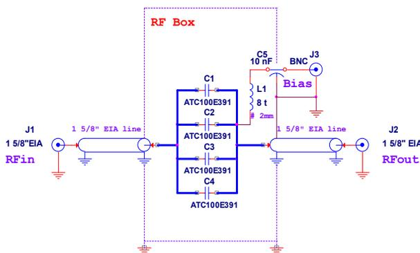
Figure 4: Electrical diagram of the final version of a 4 kW bias-T adaptor.
