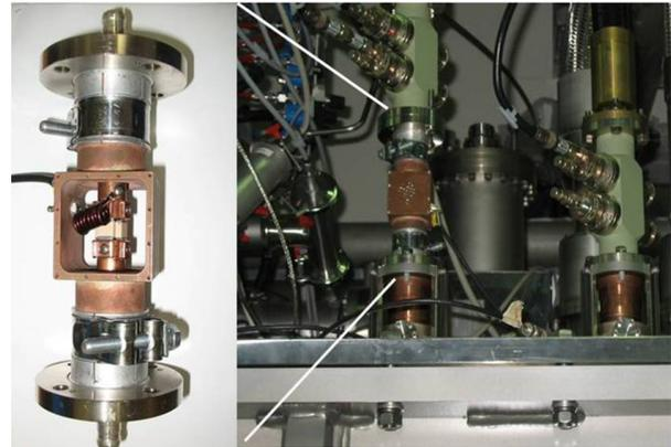
Figure 5: Left. The final version of the bias-T adaptor. Right. The adaptor installed on the PSM top.
