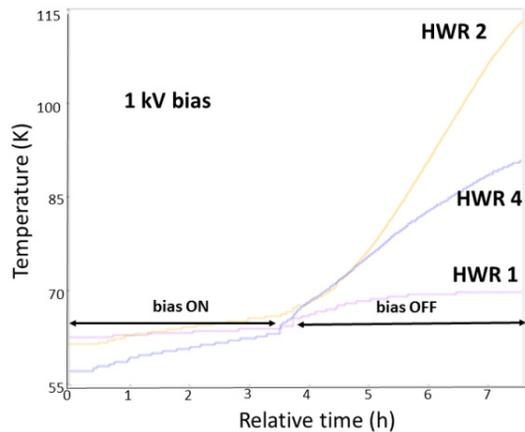
Figure 6: The effect of applying 1 kV bias on the 2<sup>nd</sup> and 4<sup>th</sup> cavities.
