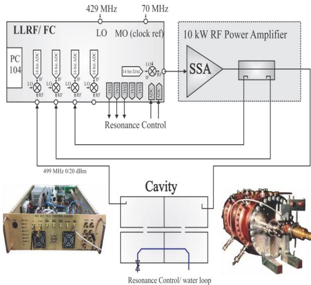
Figure 2: Single source/single cavity for extraction system
