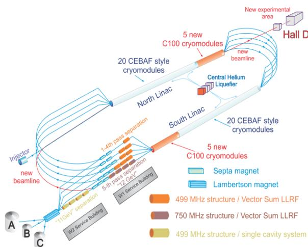
Figure 1: Layout of the 12 GeV CEBAF accelerator
