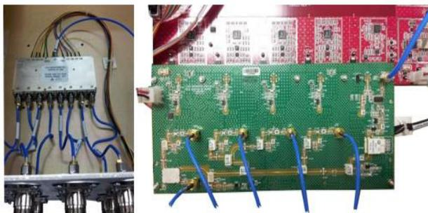
Figure 7: RF multiplexer and 748.5 MHz RF board
