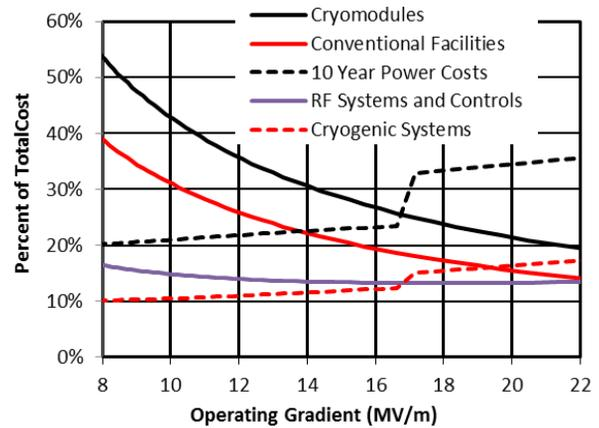
Figure 5: Relative cost breakdown for the components used in determining the cost for the XFEL-style cryomodule based linac operated at 2.0 K including building an accelerator enclosure.
