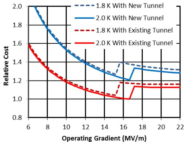
Figure 4: Relative cost of a 4 GeV linac plus 10 years of electrical power as a function of gradient and temperature for the case of using an existing accelerator enclosure and building a new accelerator enclosure.
