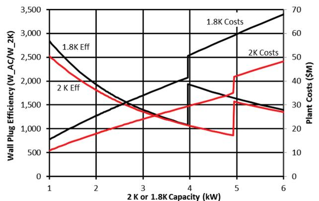
Figure 3: The wall plug efficiency and facility plant procurement costs for a helium refrigerator operated at 2.0 K and 1.8 K.
