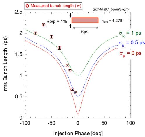
Figure 10: Measured bunch length versus beam injection phase. The solid lines show the calculation results of rms bunch length with time resolution of 0.0ps, 0.5ps, 1.0 ps.
