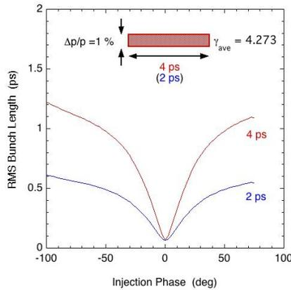
Figure 3: RMS bunch length via velocity bunching versus the beam injection phase to accelerating structure. ( $E_0 = 20\text{MV/m}$ ) Initial electron bunch has uniform charge distribution with  $\gamma_{\text{ave}} = 4.273$ ,  $\Delta p/p = 1\%$ ,  $\Delta t = 4\text{ps}$  (2ps).
