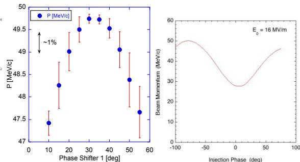
Figure 7: (Left) RF phase dependence of the beam momentum measured downstream of linac. (Right) Injection phase versus the momentum of accelerated beam (calculation).
