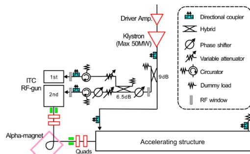
Figure 5: High power RF system for the t-ACTS injector.
