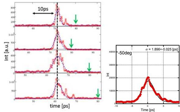
Figure 8: Measured time profile using streak camera. (Left) Samples of single shot measurement. (Right) Time profile superimposed of 30 shots.
