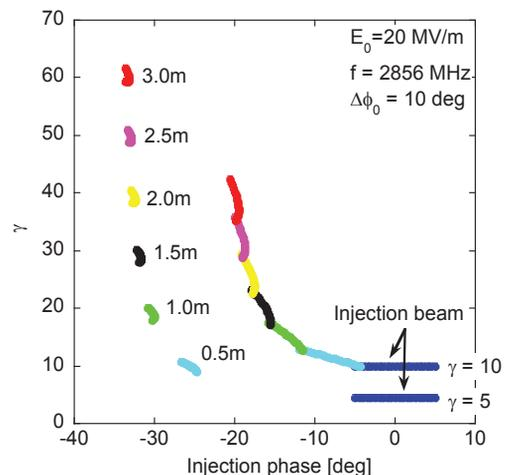
Figure 2: Equi-potential lines for the peak accelerating field  $E_0 = 20\text{ MV/m}$ . Evolutions of electron distributions injected at 0 degree are plotted with colored lines.
