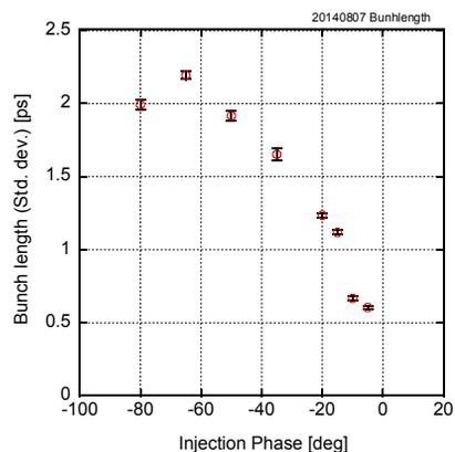
Figure 9: Measured bunch length plotted as a function of injection phase.
