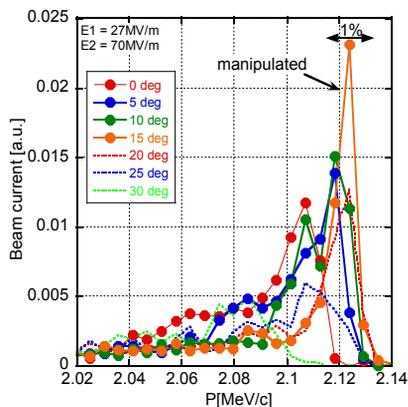
Figure 6: Measured momentum spectra for different phases of ITC RF-gun. These spectra were measured in the alpha magnet using the movable beam slit. The phase shifter set to 15 degrees (orange line) to make a spectrum with small energy spread.
