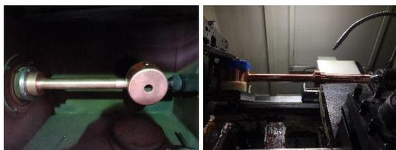
Figure 9: Electron beam welding (left) and finish machining after welding (right).
