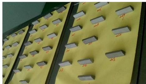
Figure 6: The magnet segments after screening.
