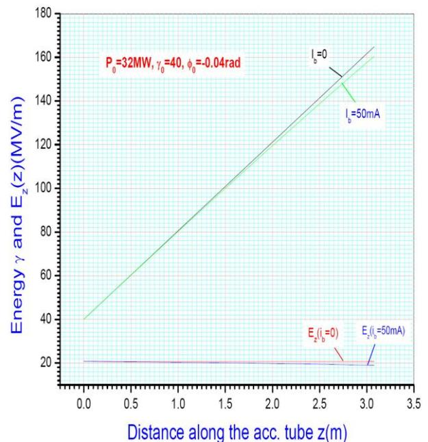
Figure 3: The field strength and energy gain in the 3m accelerating section.
