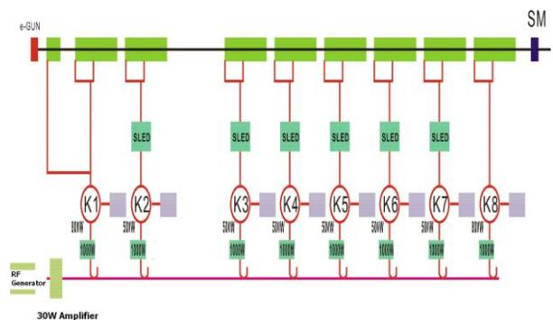
Figure2: 800 MeV electron Linac energy, phase and microwave System Layout
