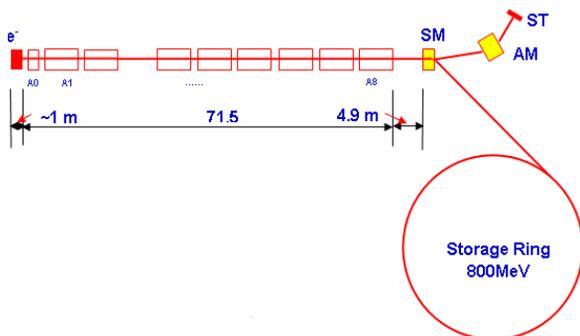
Figure1: HLS 800 MeV Linac and the electron storage ring layout
