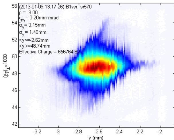
Figure 13: Vertical phase space emittance, measured at the Cornell photoinjector at a beam energy of 8 MeV.
