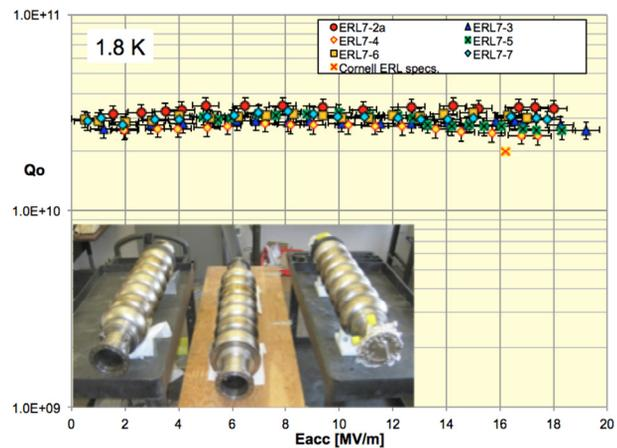
Figure 10: Quality factors of the 6 ERL cavities built at Cornell. All cavities surpass the design specifications.
