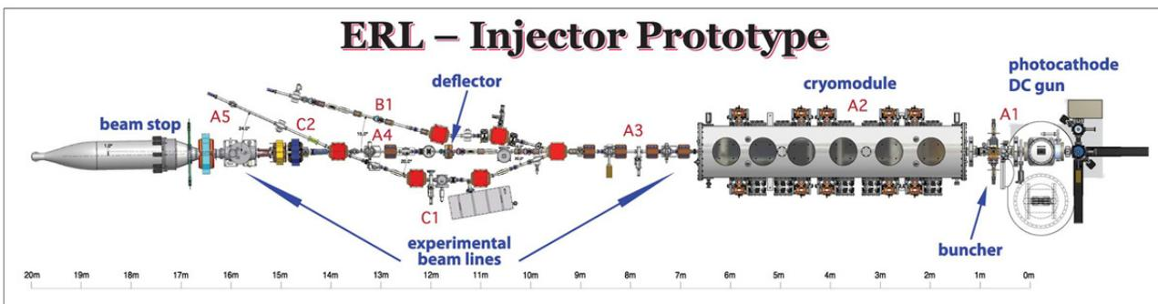
Figure 11: The Cornell ERL photo-injector, consisting of an 350 kV DC gun holding a high QE, high current photo cathode, followed by an SRF injector module based on 5 2-cell cavities, a merger section with adequate diagnostics and a beam dump.
