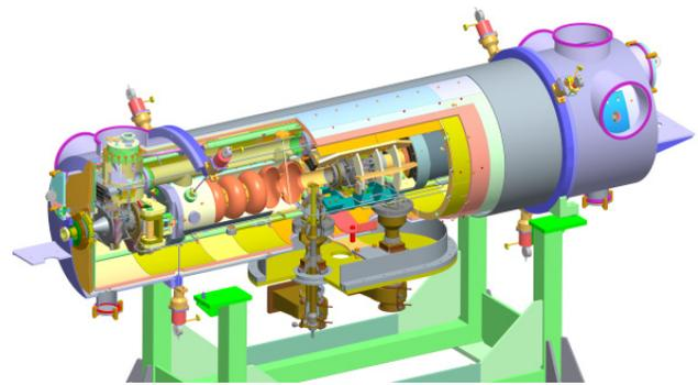
Figure 4: The international ERL cryomodule put into operation at Daresbury.
