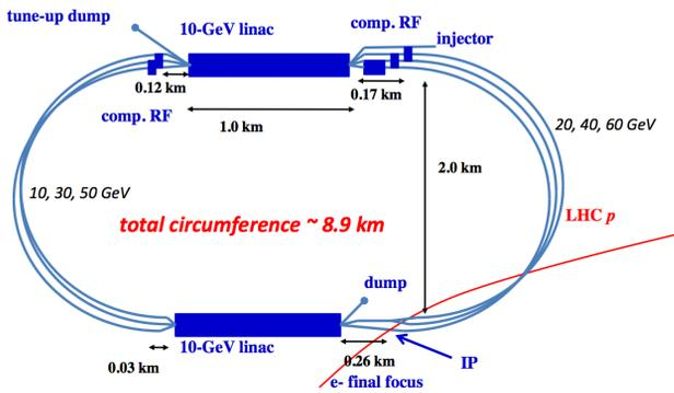
Figure 9: LHeC ERL under conceptual design at CERN.
