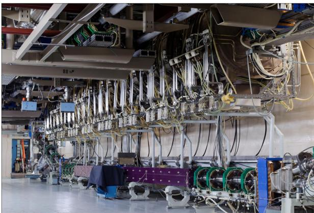
Figure 3: Energy Recovery Linac at the Budker institute. The normal conducting RF cavities are suspended from the ceiling and the return arc is bolted to the ground.
