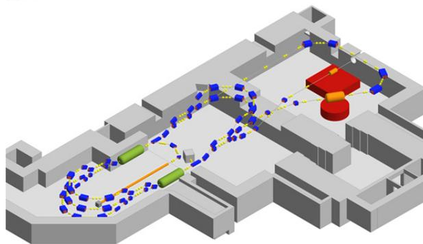
Figure 8: The planned Mesa facility at Mainz University-allowing internal nuclear physics experiments with full energy recovery as well as extracted beam operation in a recirculating linac configuration.
