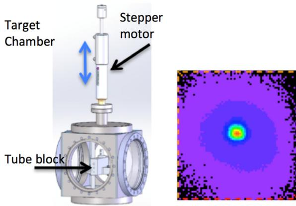
Figure 2: Set-up at JLab to testing high current ERL operation, investigating beam halo, impedance and wake field effects. The gaussian fit to the beam size yielded  $\sigma_x=50\ \mu\text{m}$ ;  $\sigma_y=52\ \mu\text{m}$ .
