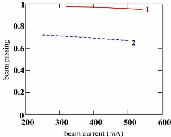
Figure 5: Beam passing vs beam current for two regimes: 1—with applying optimized additional RF voltage to the grid-cathode gap; 2—without additional RF voltage.
