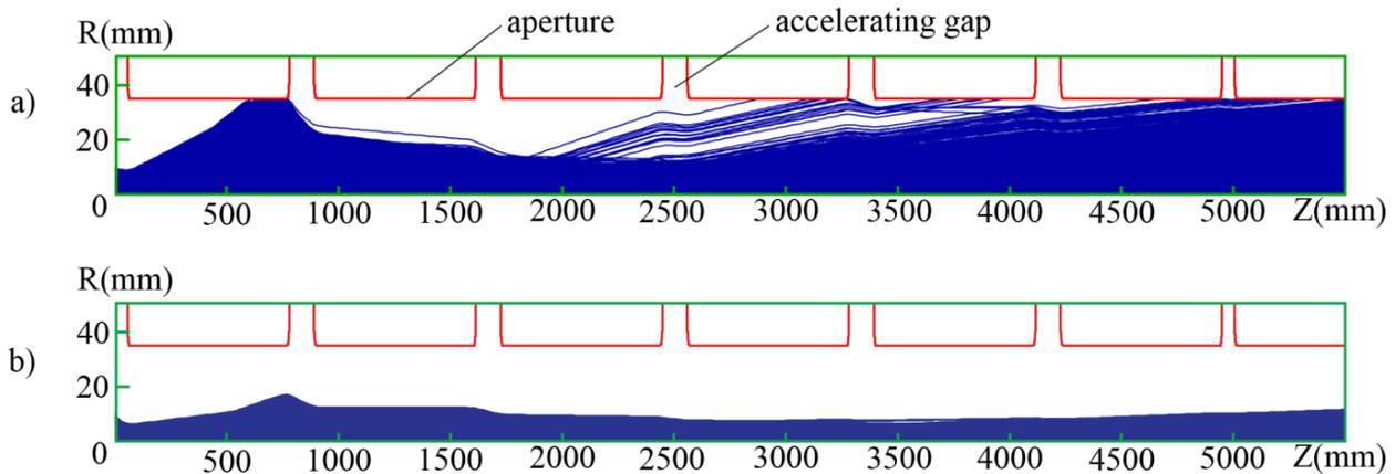
Figure 7: Trajectories of electrons in ILU-14 accelerating structure: a) for 7.5 MeV regime; b) for 10 MeV regime.
