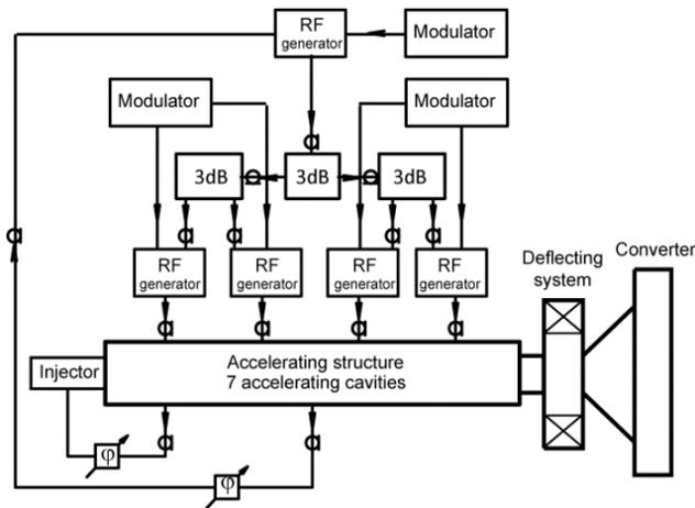
Figure 1: ILU-14 block diagram.
