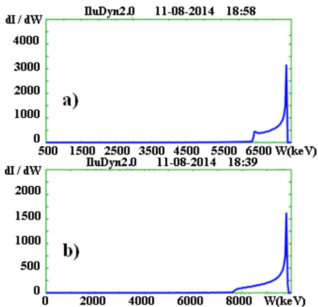
Figure 8: Electron energy spectrums for 7.5 MeV (a) and 10 MeV (b) regimes.
