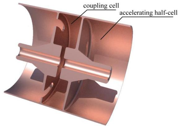
Figure 3: Accelerating structure period (section view).
