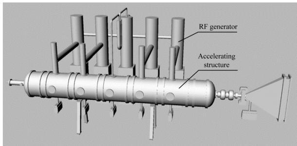
Figure 2: ILU-14 accelerator 3D view.
