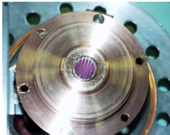
Figure 4: Grid-cathode unit of the RF gun for ILU-14 accelerator.
