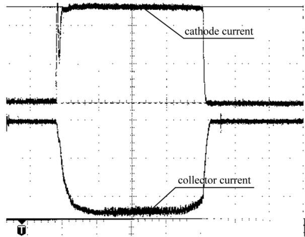
Figure 6: Oscillograms of the cathode and collector currents.
