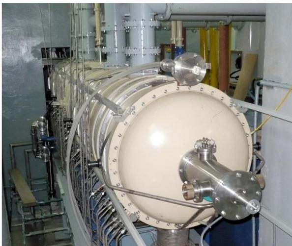
Figure 9: ILU-14 accelerator in radiation shielded room of the sterilization Complex.
