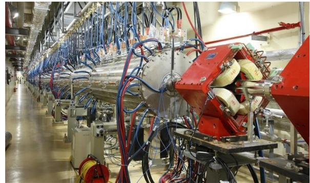
Figure 2: 100 MeV proton linear accelerator
