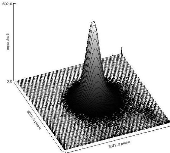
Figure 6: Beam profile at the target room
