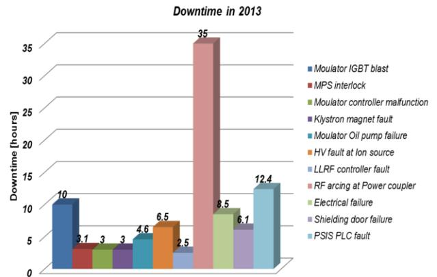
Figure 8: Down time of each component
