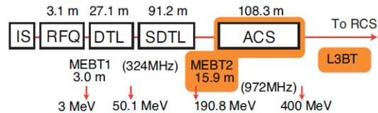
Figure 1: The configuration of the energy upgraded J-PARC linac.
