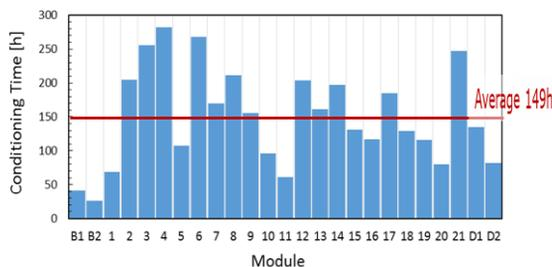
Figure 5: Conditioning time for each ACS module to achieve a specified power level at a pulse length of 600  $\mu$ sec.
