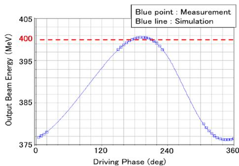
Figure 7: Phase scan result at the last ACS module.
