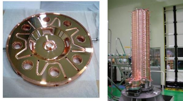
Figure 3: ACS half-cell disk (left) and stacked view of the disks before brazing (right).
