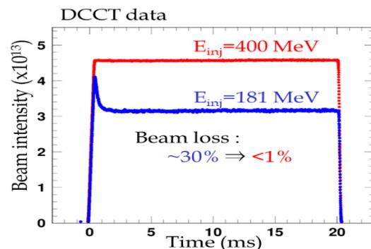
Figure 9: Beam intensity in the RCS for 400 MeV and 181 MeV injection cases (beam current 25 mA, no injection painting).
