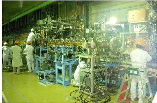
Figure 10: New ion source and RFQ in the linac tunnel. (August 2014)
