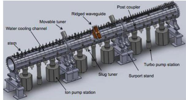
Figure 2: general drawing of DTL tank.
