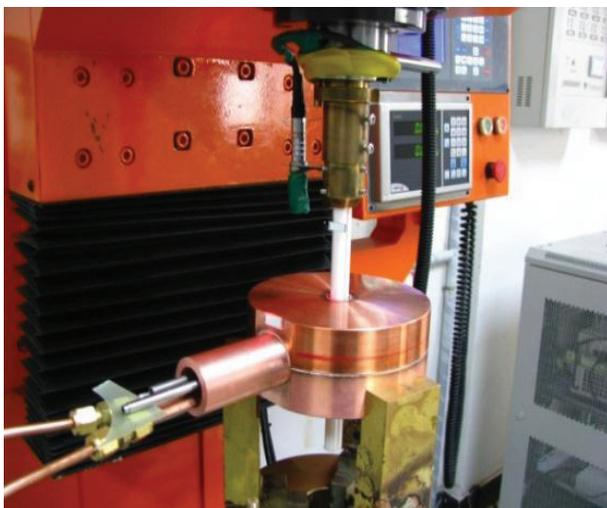
Figure 10: rotating coil measurement
