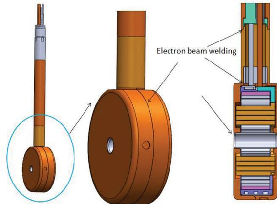
Figure 6: View of a typical Drift tube.
