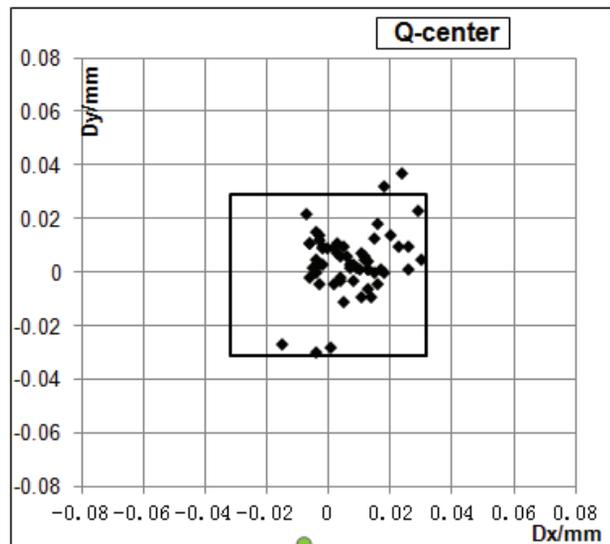
Figure 11: Deviation of the mechanical centre from magnetic field centre.
