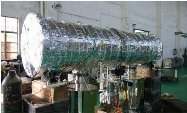
Figure 5: bake out of DTL tank.
