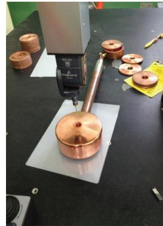
Figure 7: mechanical dimension measuring by three-coordinate measuring machine.
