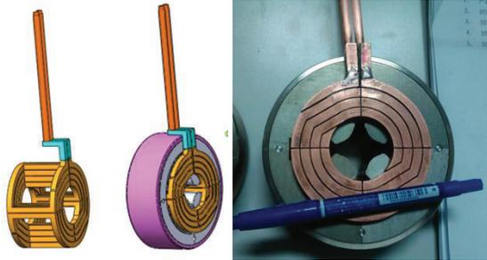
Figure 9: View of hollow coil and magnet.
