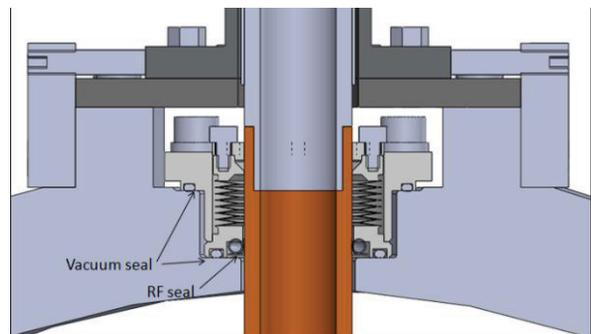
Figure 8: schematic layouts of DT stem assembly.
