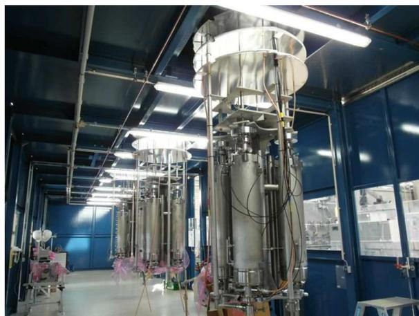
Figure 1: XFEL cavities installed into the insert.
