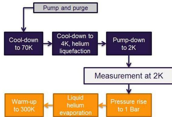
Figure 6: Cryogenics operation sequence for cryomodule test stand.
