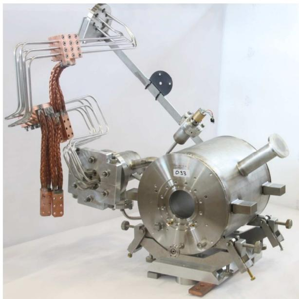
Figure 2: Superconducting magnet with current lead
