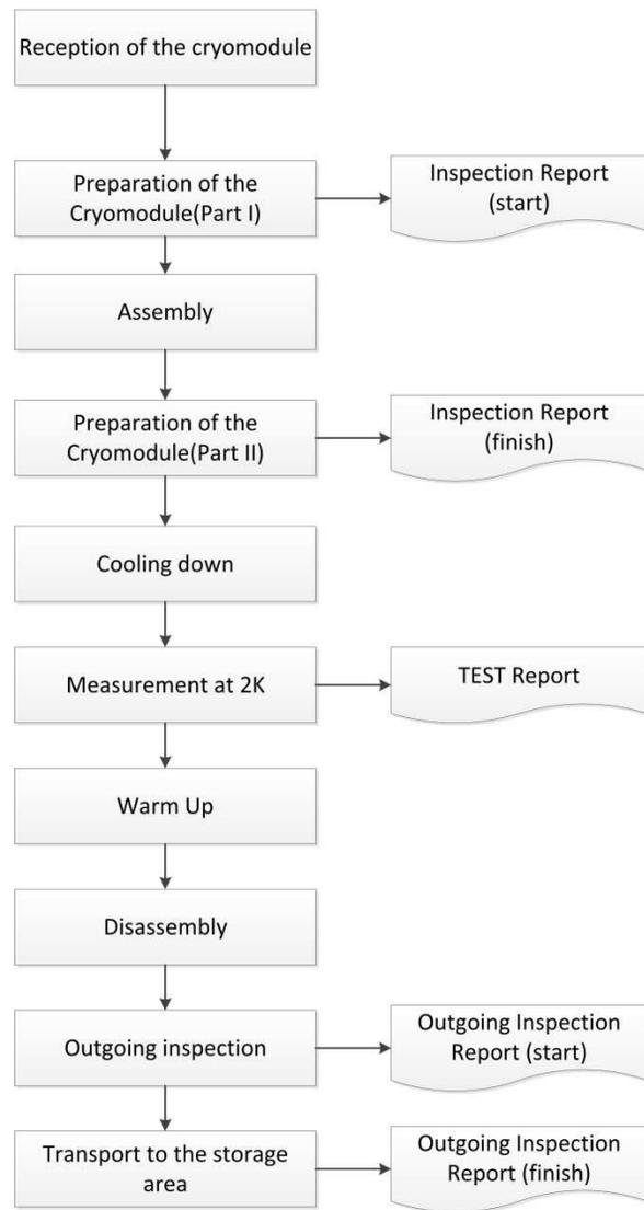
Figure 4: Cryomodule test main flow diagram.
