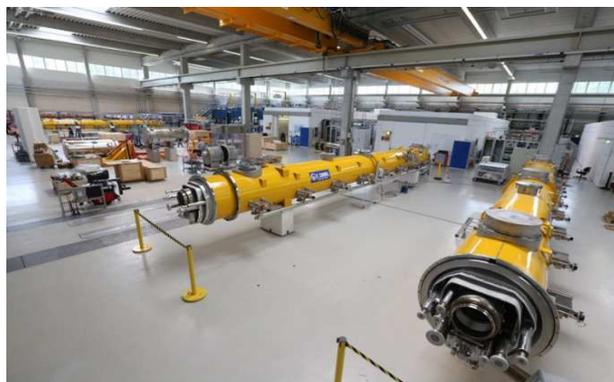
Figure 3: Inside view of the AMTF hall – cryomodules.
