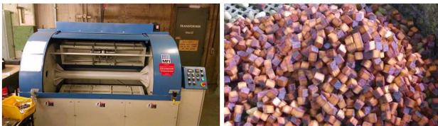
Figure 6: Centrifugal barrel polish machine loaded with Nb<sub>3</sub>Sn cavity (left); and polishing media after 4.5 hours (right).
