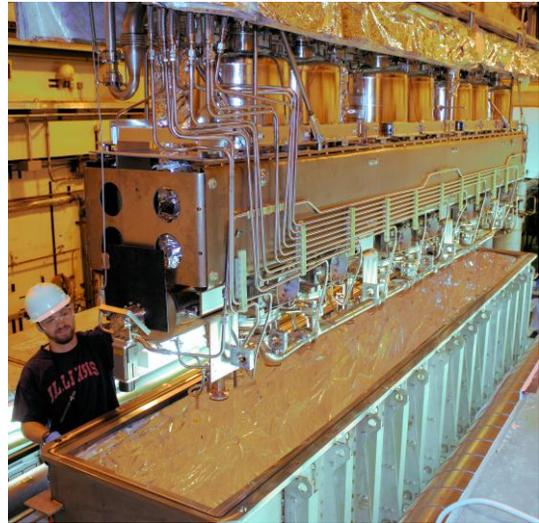
Figure 3: Test fitting the cavity string assembly in the cryostat vacuum vessel
