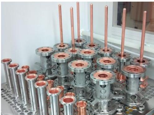
Figure 6: ATLAS 4 kW RF power couplers
