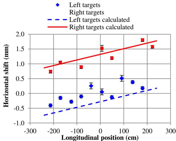
Figure 4: Horizontal shifts of crosshair targets on evacuation of the cryomodule and the subsequent cooldown.
