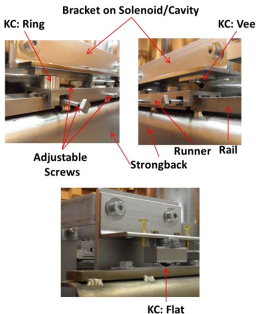
Figure 2: Pictures of the kinematic-alignment hardware: the top two ones show one side of the strongback and the bottom one shows the other side.
