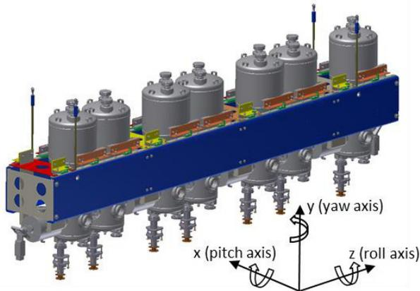
Figure 1: 7 cavities and 4 solenoids mount on the strongback (blue) with their own kinematic-alignment hardware (orange for cavity and yellow for solenoid). 4 supporting hangers are hung on the cryomodule lid which is transparent in this model view.
