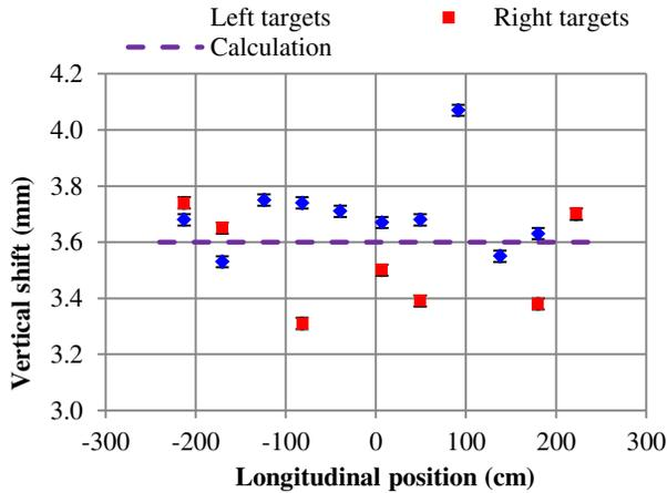
Figure 3: Vertical shifts of crosshair targets on evacuation of the cryomodule and the subsequent cooldown. The cavity string configuration is S-C-C-S-C-C-S-C-C-S-C from the left end, where S denotes solenoid and C denotes cavity.
