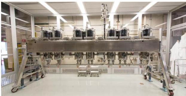
Figure 4: String of seven superconducting resonators and four solenoid magnets after completion of clean assembly.
