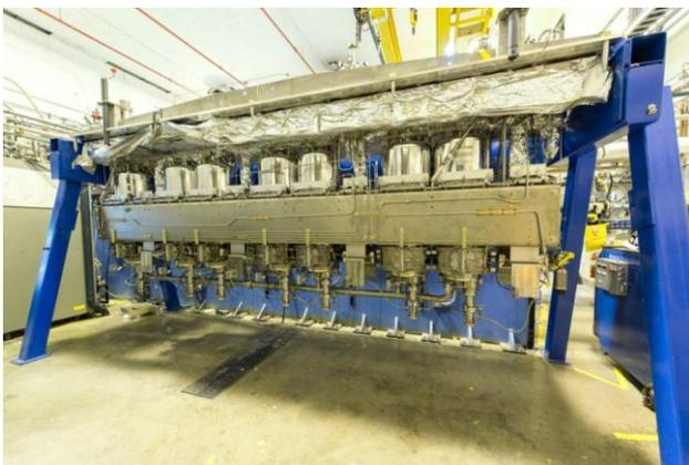
Figure 5: Cold mass assembly is ready to load into the cryostat vacuum vessel.
