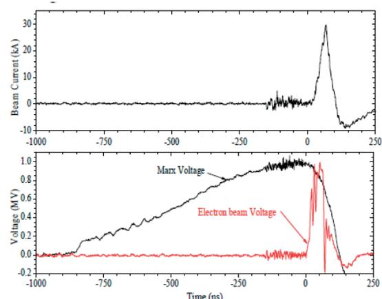
Figure 2: Electron beam current (above) and Marx voltage and Diode Voltage for KALI 30 GW system.
