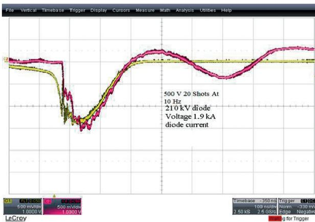
Figure 4: LIA 400 operation at 10 Hz repetition rate.
