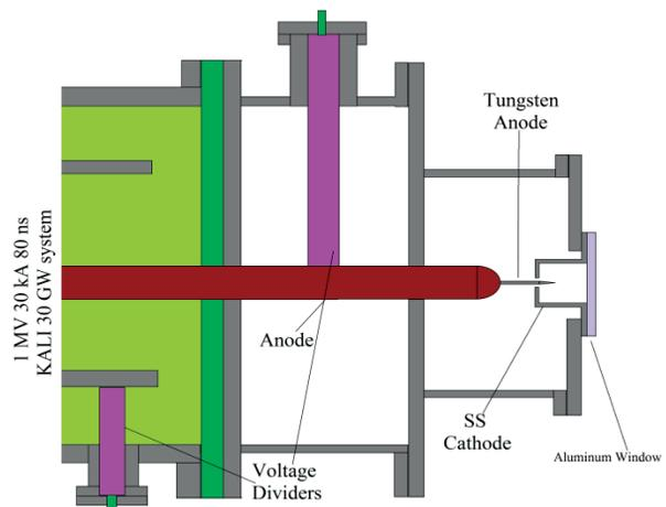
Figure 6: The schematic diagram of a FXR diode.
