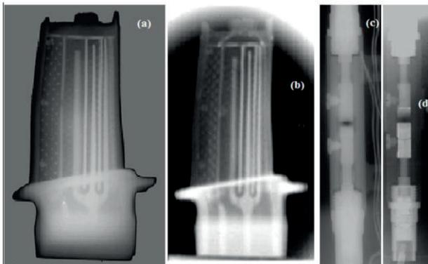
Figure 7: Radiography images of (a) turbine blade recorded by FXR and (b) by neutron radiography, (c) INSAT cable cutter with FXR and (d) with neutron radiography.
