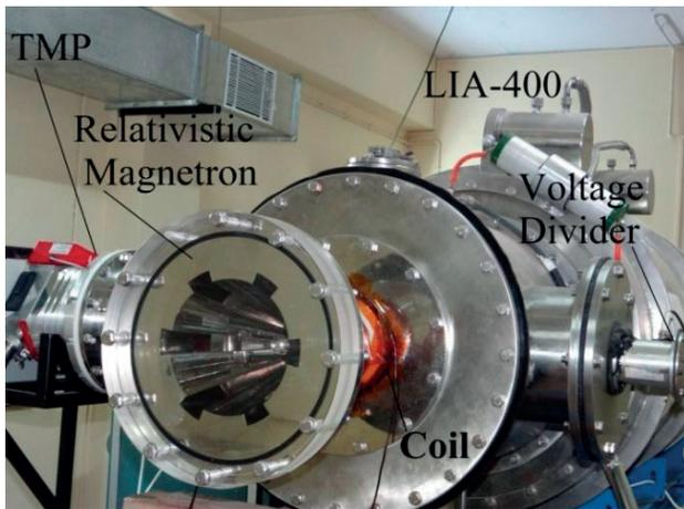
Figure 3: LIA 400 System with Relativistic magnetron
