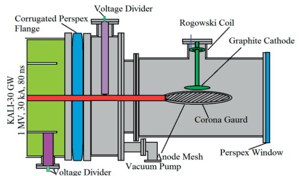
Figure 5: The schematic of a reflex triode Vircator.
