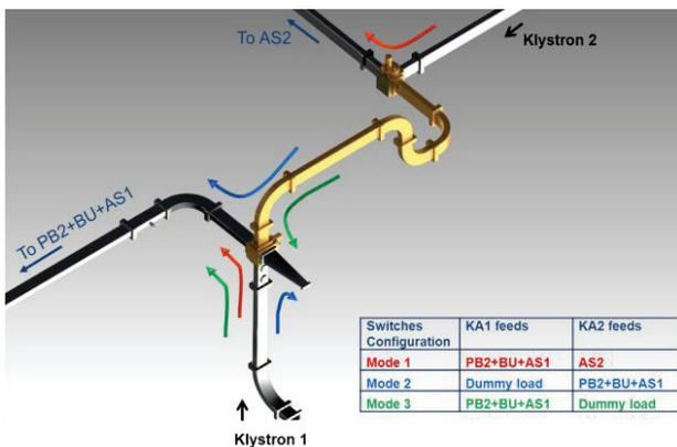
Figure 7: The two WR284 waveguide circuits are now connected by means of two switches manufactured by Sector-Microwave. They offer three modes of operation.
