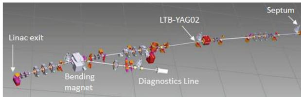
Figure 3: Schema of the Linac To Booster transfer line (LTB) and the Linac Diagnostics line (LiDia).
