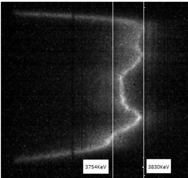
Figure 2: time-resolved spectrum of the electron beam at accelerator input
