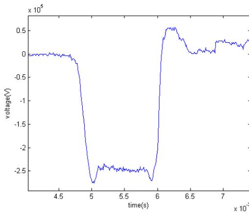
Figure 3: voltage pulse shape at an accelerating cell
