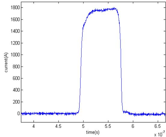
Figure 4: beam current output pulse shape
