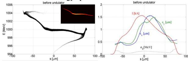
Figure 4: Beam bunch properties before the modulator for HGHG. Longitudinal phase space (left), Current profile, slice emittances and slice energy spread (right).
