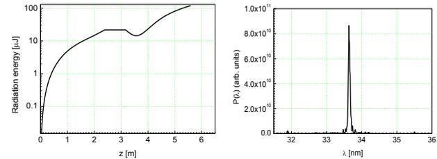
Figure 7: Radiation energy along the radiator (left) and the spectrum (right).
