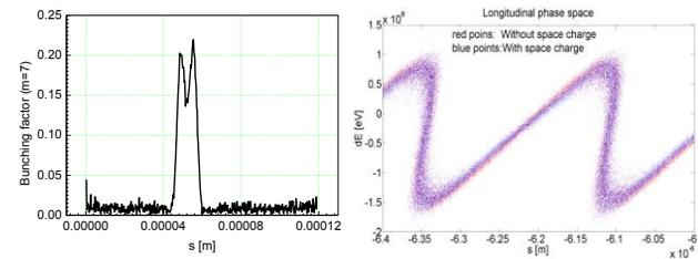
Figure 6: Bunching factor (left) and longitudinal phase space (right) at the entrance of the radiator.
