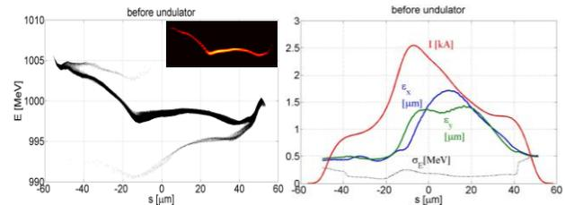
Figure 3: Beam bunch properties before SASE undulator. Longitudinal phase space (left), Current profile, slice emittances and slice energy spread (right).
