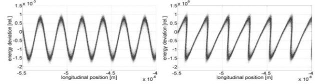
Figure 5: Longitudinal phase spaces after the modulator (left) and after the dispersive chicane (right).
