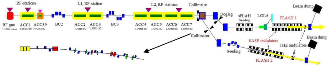
Figure 1: Schematic layout for FLASH facility and the extraction arc of FLASH2.
