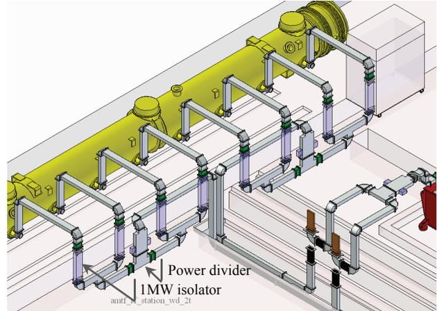
Figure 1: 3D-view of the AMTF waveguide distribution.
