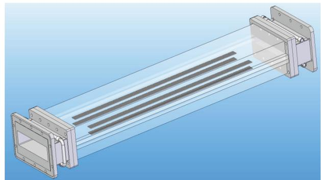
Figure 2: View of the S.P.A.FERITE 1 MW isolator.
