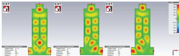
Figure 3: RF power distribution depending on the phase shifter piston position
