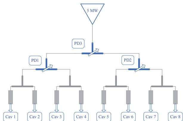
Figure 4: Schematic of the power distribution system.
