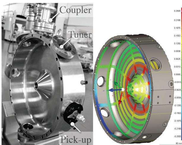
Figure 3: **Left:** Picture of the AISI 304 buncher prototype after machining. **Right:** 3D metrology corresponding to *Body* part of the prototype. Colorbar scale represents measured deviation respect to drawings values, in mm.
