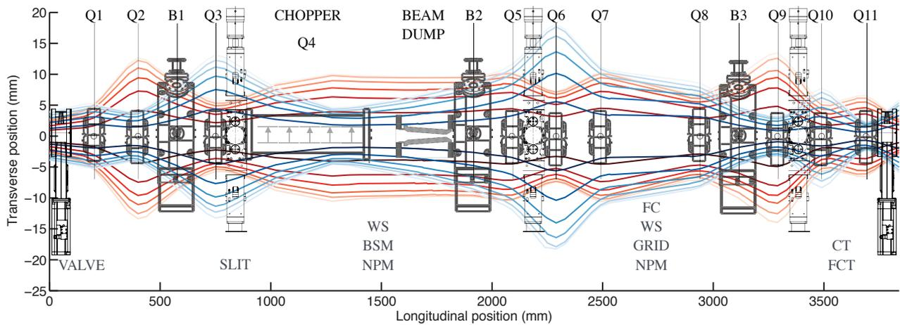
Figure 2: 2014 Layout proposed for the ESS MEBT; comprised of 11 quadrupoles 3 bunchers and 3 collimators [4]. Power density contours for x (red) and y (blue) are represented from dark ( $10^3$  W) to light ( $10^{-2}$  W) beam power contour lines extracted from TRACEWIN. Both axis are expressed in mm.
