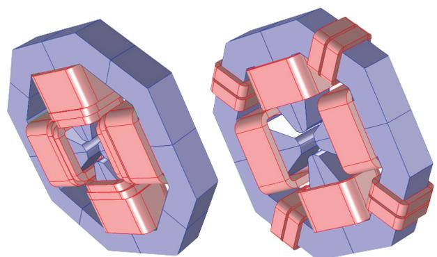
Figure 4: 3D models of proposed Steerer Coils In (**Left**) and Steerer Coils Out (**Right**). Coils are represented in red.
