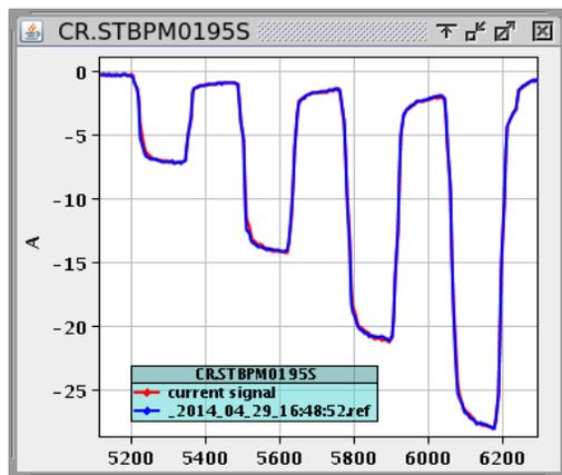
Figure 1: Beam current vs. time (ns), showing the four-fold increase during beam combination in the combiner ring. The two overlapping traces (red and blue) were taken on two different days, with identical machine settings.
