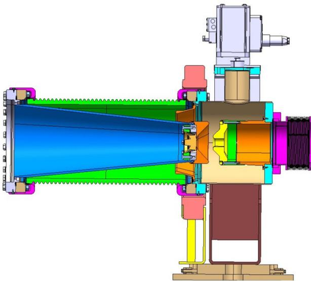
**Figure 5:** Mechanical design of the thermionic electron source consisting of a conical structure (blue) holding the cathode (orange) inserted into the insulation ceramics (green) and a separate anode (yellow) chamber.
