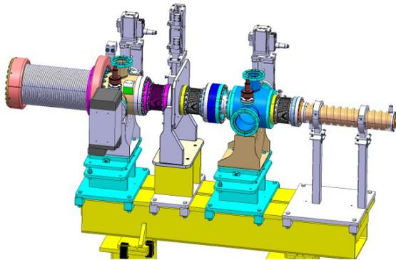
**Figure 4:** Mechanical layout of the gun test beam line including the high voltage ceramic (left), pumping ports, a current transformer and a beam dump.
