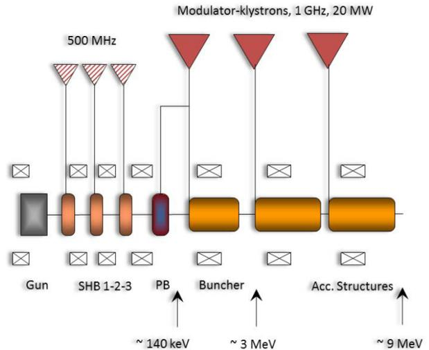
**Figure 1:** Layout of the CLIC drive beam injector front end. From left to right: Thermionic gun, 500 MHz sub-harmonic bunchers, 1 GHz pre-buncher, 1 GHz travelling wave buncher and two 1 GHz accelerating structures.
