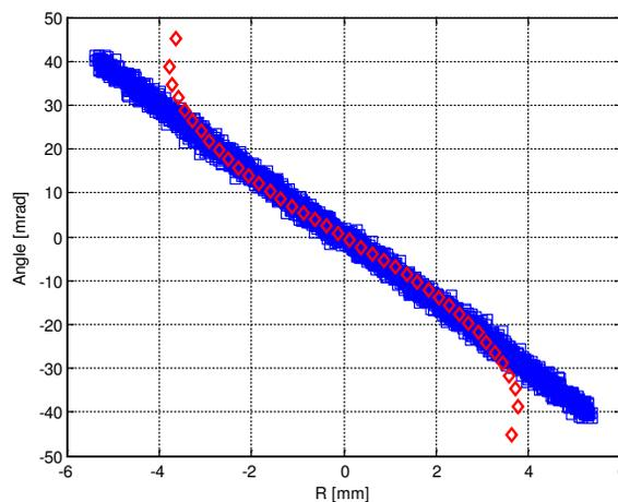
**Figure 3:** Comparison of the phase space at the exit of the gun as simulated by EGUN (red) and MAGIC (blue). This simulations are for a 5 A beam from a 10 mm radius planar cathode, evaluated at the exit of the anode.
