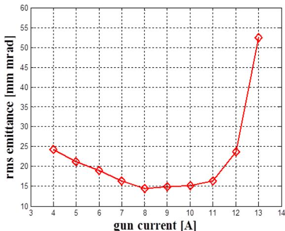
**Figure 2:** Current dependence of the emittance for the 8 mm cathode in the CTF3 gun.
