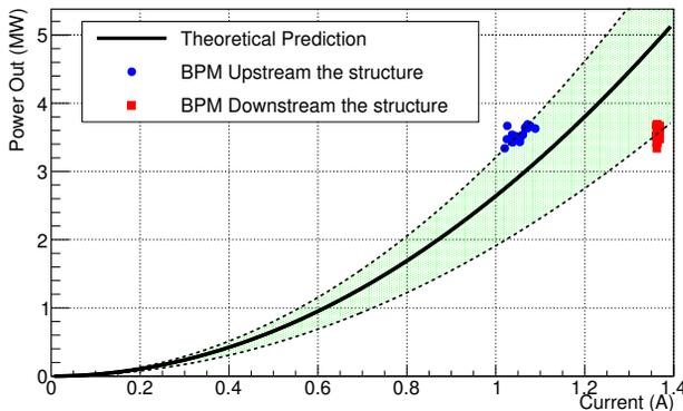
Figure 5: Steady-state forward RF output power of the accelerating structure as function of beam current, for the theoretical prediction and for experimental results (shadow area) bounded by measurements of current upstream and downstream the accelerating structure.
