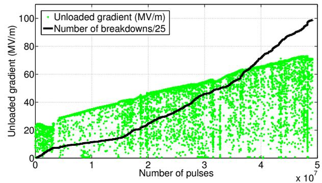
Figure 6: Evolution of gradient (green) and accumulated breakdowns (black) for the dogleg structure.
