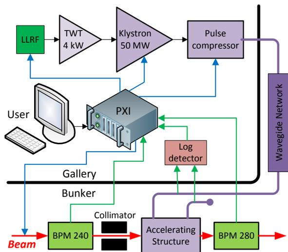
Figure 3: Simplified scheme of the hardware installation, control and acquisition system.
