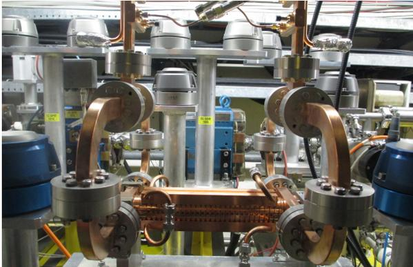
Figure 2: T24 structure installed in the CTF3 Dogleg line.
