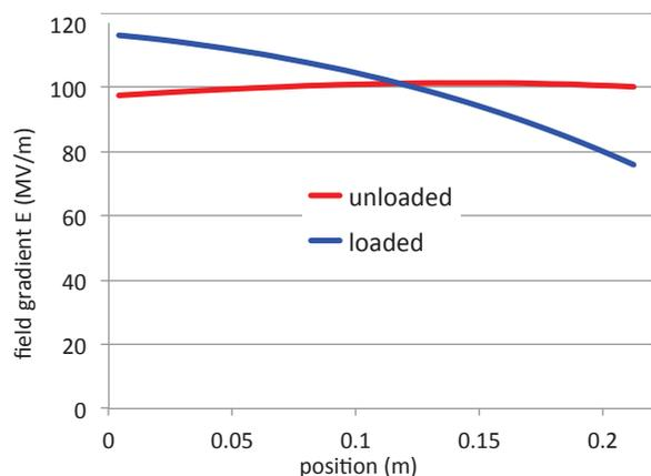
Figure 1: Longitudinal field gradient profile for an unloaded (red line) and 1.2 A of beam loaded (blue line) CLIC travelling wave structure at 100 MV/m average gradient.
