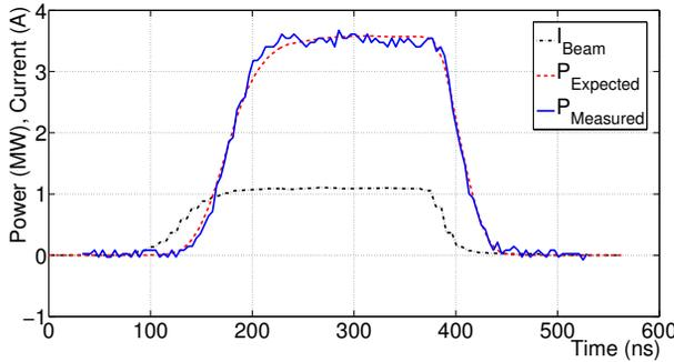
Figure 4: Forward RF output power of the accelerating structure calculated from the measured beam current profile along the pulse together with measurement (scaled in power level).
