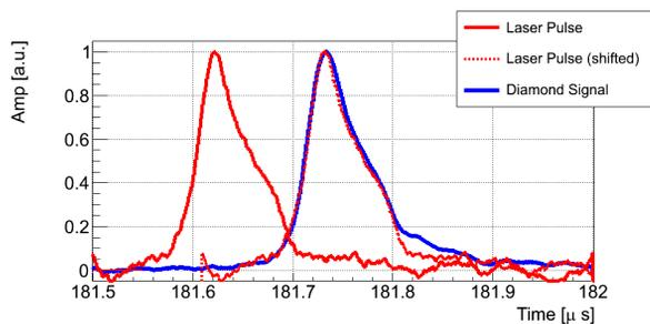
Figure 5: Zoom on one of the diamond signals of Fig. 4, compared to the corresponding laser pulse (as recorded by a scope and shifted in time to see the overlap with the diamond signal).
