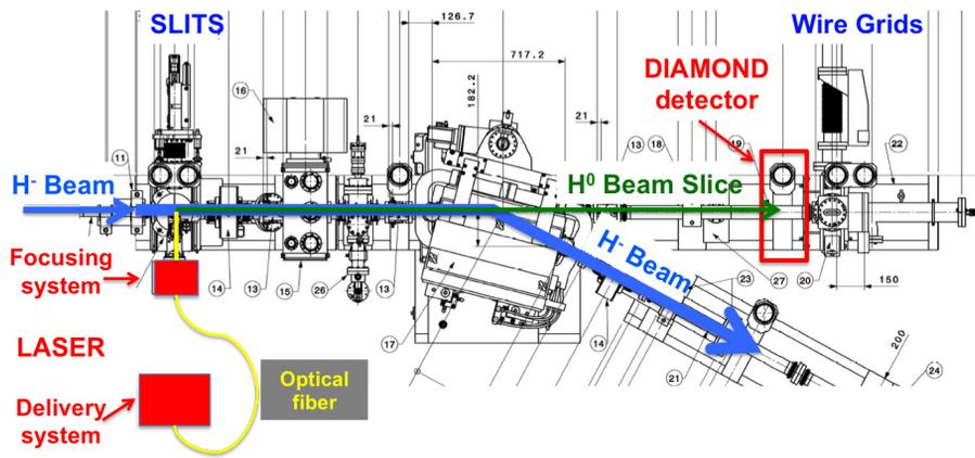
Figure 2: Layout of the 3 MeV diagnostics line as it was installed after the MEBT, including the operational emittance meter (slit and grids) and the prototype laser-diamond system.
