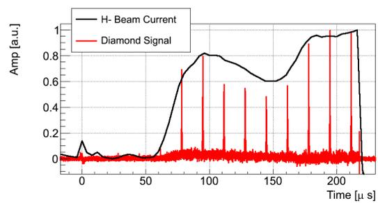
Figure 7: Comparison between the diamond and the beam current transformer upstream of the laser during the very first test at 12 MeV.
