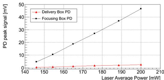
Figure 3: Photo diodes peak signals as a function of average laser power (with 60 kHz repetition rate and 10 ms amplification period).
