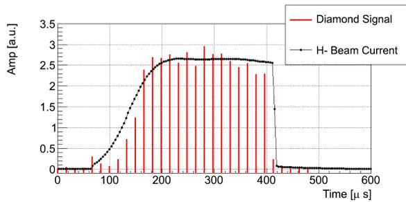
Figure 4: Signal from a single diamond detector channel sampling the  $H^0$  particles for a given laser position, as function of time along the  $H^-$  beam pulse. This is compared to the beam current measured with a beam current transformer upstream the laser station.
