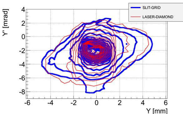
Figure 6: Contour plots resulting from a slit-grid and laser-diamond scans at 3 MeV.
