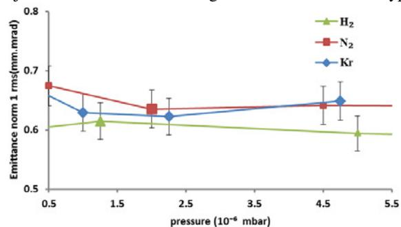
Figure 4 Emittance vs injected partial pressure for H<sub>2</sub>, Kr and N<sub>2</sub>.
