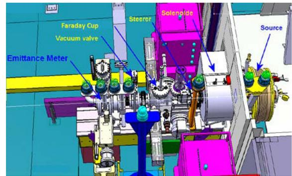
Figure 1: Experimental Setup Distance between the emittance meter and source 1.308 m
