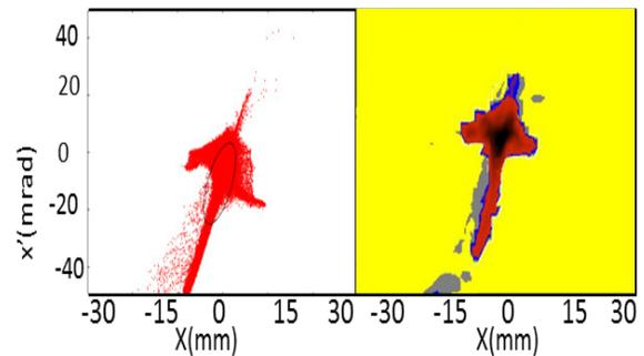
Figure 3: Beam phase space with two components. Simulation (left), measurement (right).
