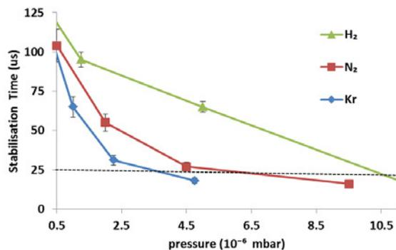
Figure 5: Measured decay time of the beam size of the partial pressure for H<sub>2</sub>, Kr and N<sub>2</sub>. The dot line shows the required pressure to get a stabilisation in 25  $\mu$ s.
