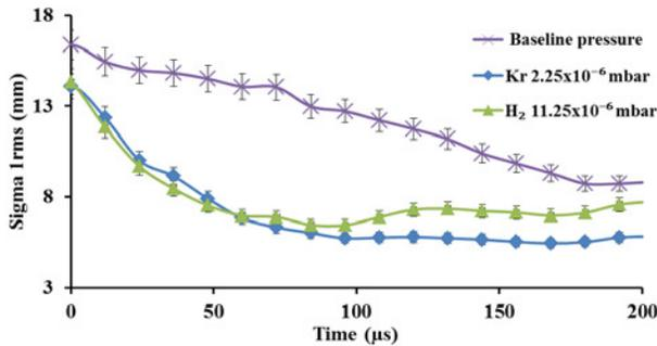
Figure 2: Beam size measured at the emittance meter as a function of time, for the baseline pressure and two different injected gases.
