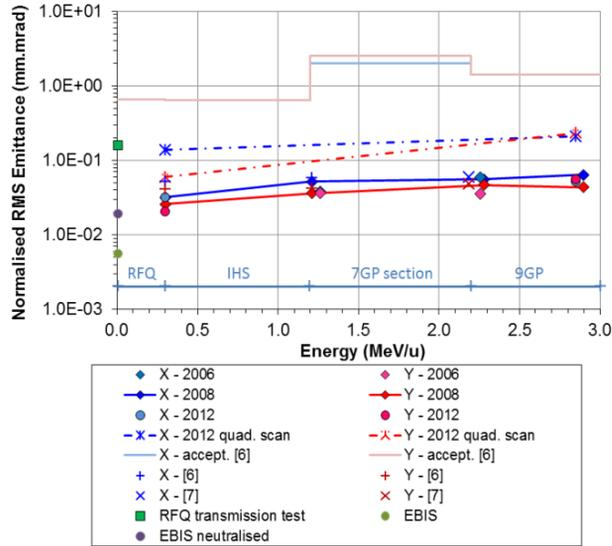
Figure 5: Summary of transverse emittance measurements at REX-ISOLDE. Design emittance and measurements from the REX-ISOLDE commissioning are shown for comparison [6] [7]. The geometrical acceptance is also indicated.
