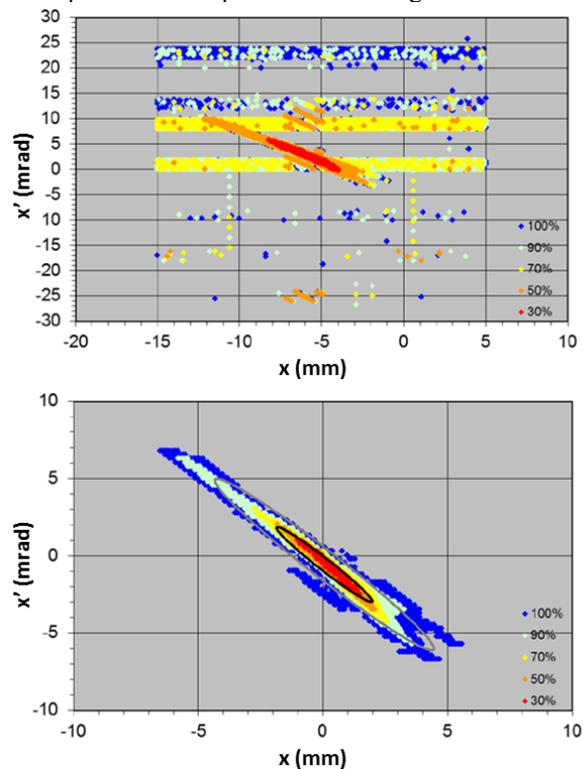
Figure 1: Emittance scan of a 2.85 MeV/u beam of Ne5+, raw data (top), emittance plot after background suppression (bottom)
