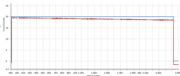
Figure 2: Current pulse from the ACCT before and after FPGA processing.
