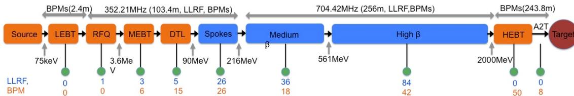
Figure 1: BPM and LLRF system number distribution at ESS.
