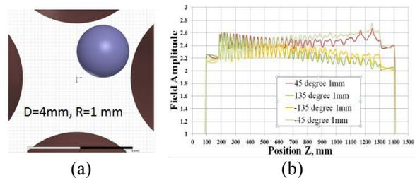
Figure 9: (a) bead 1 mm off axis inside the tips aperture of the RFQ, (b) electric field measured off axis.
