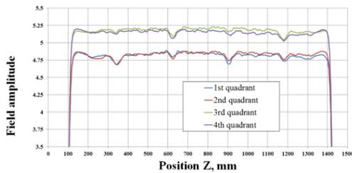
Figure 6: quadrant bead pull, R= 30 mm, bead diameter= 9.5 mm, visually aligned on the end plates.
