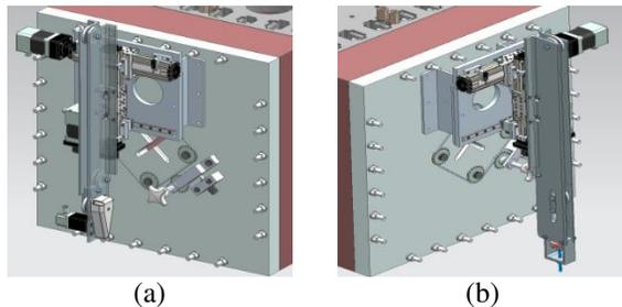
Figure 3: (a) bead line drive motor plate, (b) load cell support plate.
