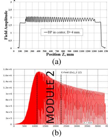
Figure 8: RFQ Ez field on axis measured with bead pull (a) and simulated (b).
