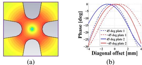
Figure 4: (a) transverse section electric field distribution, (b) phase vs diagonal offset string scan data.
