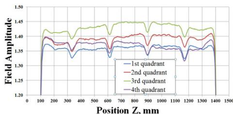
Figure 7: quadrant bead pull data, R= 30 mm, bead diameter= 4 mm, aligned on electric axis.
