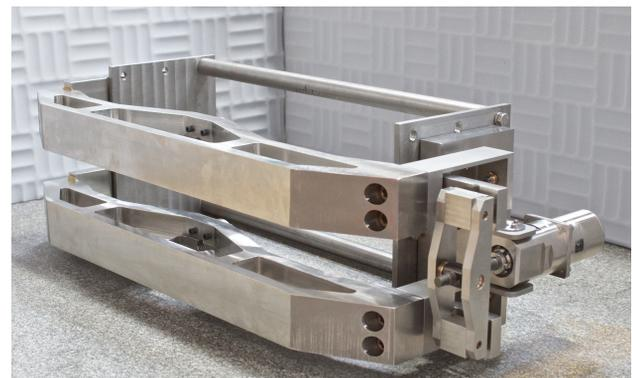
Figure 6: First prototype of the SSR1 double lever tuner.
