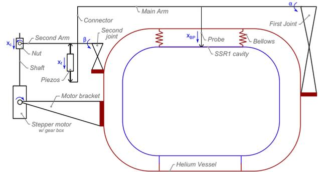
Figure 1: Schematic for the tuning system showing the cavity inside the helium vessel.
