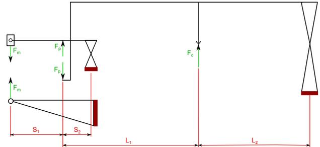
Figure 2: Scheme of force acting on the Tuner.  $L_1 = 350$  mm,  $L_2 = 350$  mm,  $S_1 = 67$  mm,  $S_2 = 30$  mm
