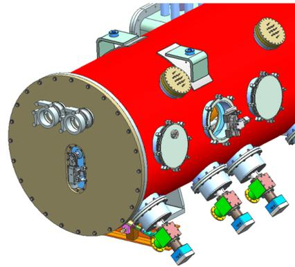
Figure 5: Access ports to the removable cartridge.
