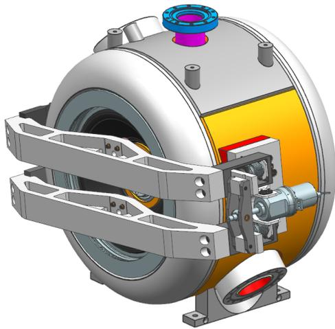
Figure 3: 3D model of the Tuner assembled on the SSR1-G3 cavity.
