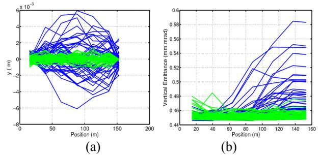
Figure 3: (a) Beam trajectories and (b) normalized rms vertical beam emittance for 50 seeds before (blue) and after (green) applying 1-1 correction algorithm.
