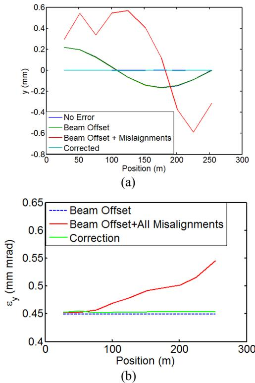
Figure 5: (a) Average beam trajectory and (b) average beam emittance in L3 section.
