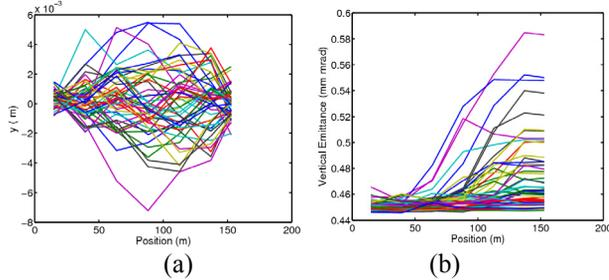
Figure 1: (a) Beam vertical trajectories and (b) normalized rms vertical emittances for 50 seeds of applying all nominal misalignments to the L2 section.
