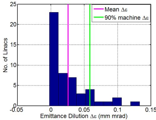
Figure 2: Resulting emittance growth distribution for 50 seeds. 90% and mean emittance growth are shown in green and magenta respectively.
