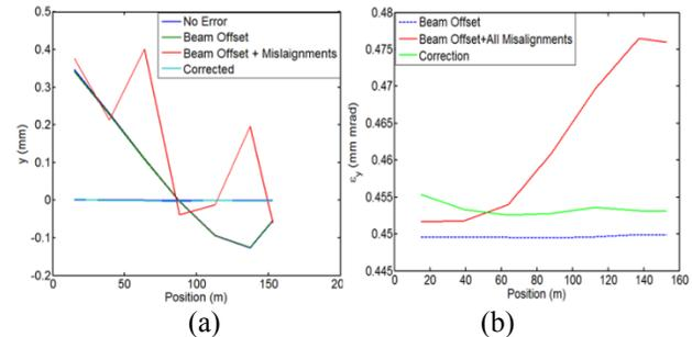
Figure 4: (a) Average beam trajectory and (b) average beam emittance in L2 section.
