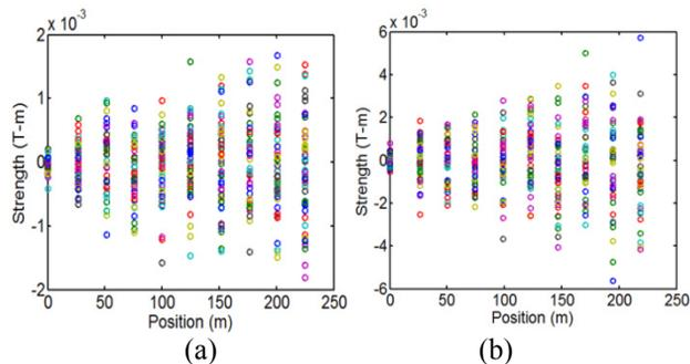
Figure 6: Distribution of corrector fields in L3 section for all 50 seeds with (a) nominal misalignment errors (b) twice of nominal misalignments errors.
