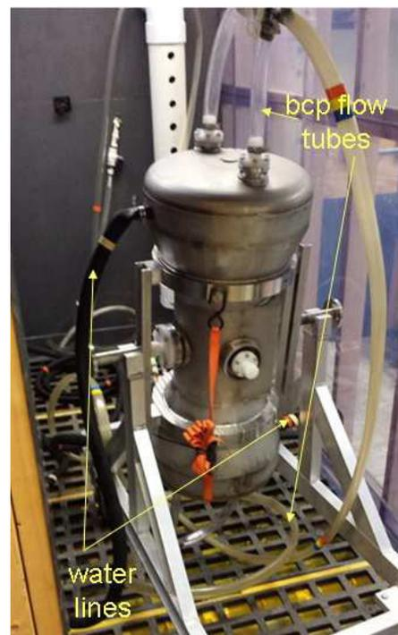
Figure 7: Buffered chemical polishing setup.
