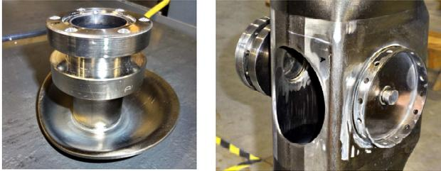
Figure 3: Cavity beam port with flanges (left) and central part (right).
