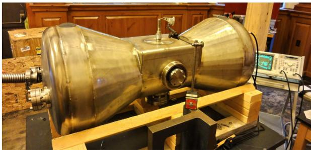
Figure 9: Helium vessel leak check setup.
