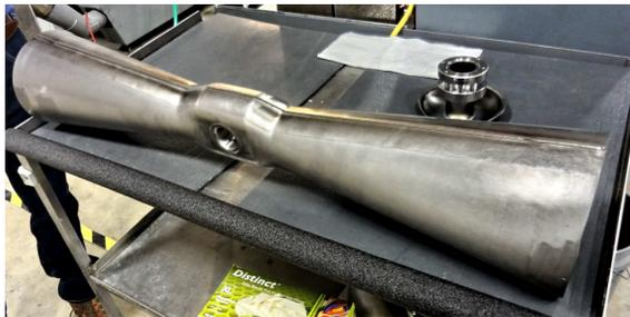
Figure 4: cHWR central electrode.
