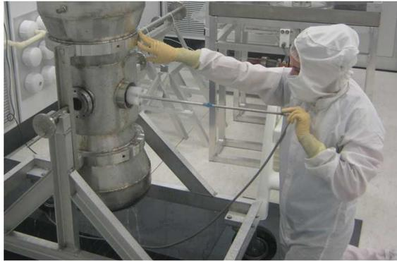
Figure 8: High-pressure water rinse setup.
