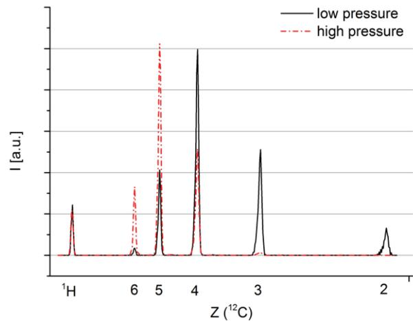
Figure 5: Gas stripper spectrum of the  $\text{CH}_3^+$ -beam from the HSI. Above a threshold (black) the proton beam intensity is independent on the  $\text{N}_2$ -target density, while the carbon beam could be optimized for higher Z (red).
