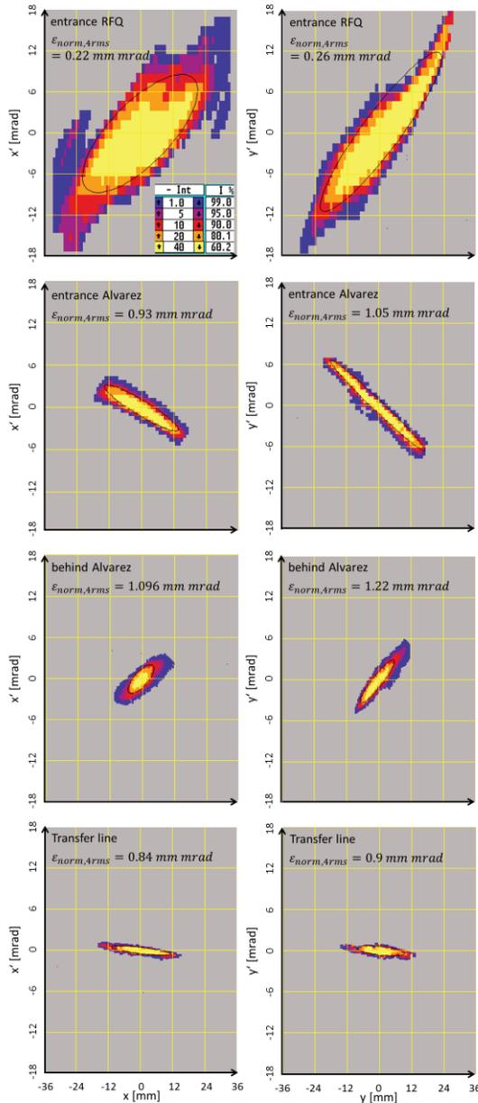
Figure 6: Measured high current proton beam emittance.
