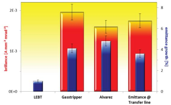
Figure 7: High current emittance growth and beam brilliance measurements along UNILAC.
