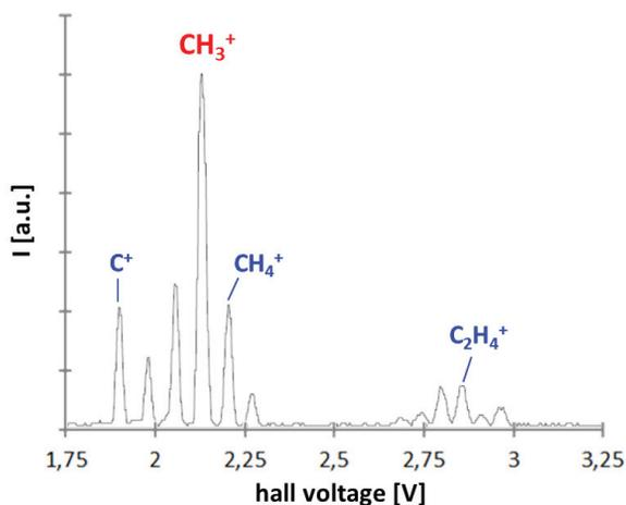
Figure 4: Optimized mass spectrum for  $\text{CH}_3^+$ -operation with the MUCIS.
