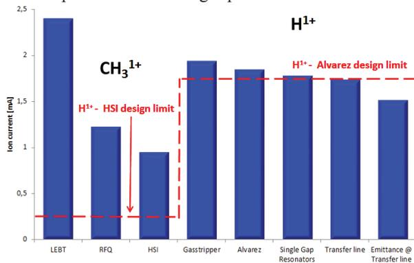
Figure 3: Measured beam current along UNILAC and transfer line to the SIS18; proton design limit was reached in the post stripper section.
