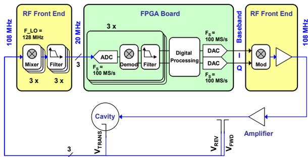
Figure 3: Signal processing in the Ampegon d-LLRF system [7].
