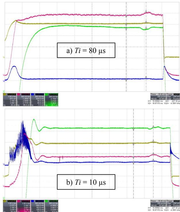
Figure 4: Measured demodulated RF signals at different settings of the FPGA based PI controller (see text). CH1 (yellow): forward power 300 W pre-driver, CH2 (red): forward power to accelerator cavity, CH3 (blue): reverse power, CH4 (green): cavity amplitude (zoom, 0.2 V/div at 5 V signal amplitude). CH3 is measured by different RF detectors in plots a) and b). The right vertical line cursor marks the centre position of the 100  $\mu\text{s}$  beam pulse.
