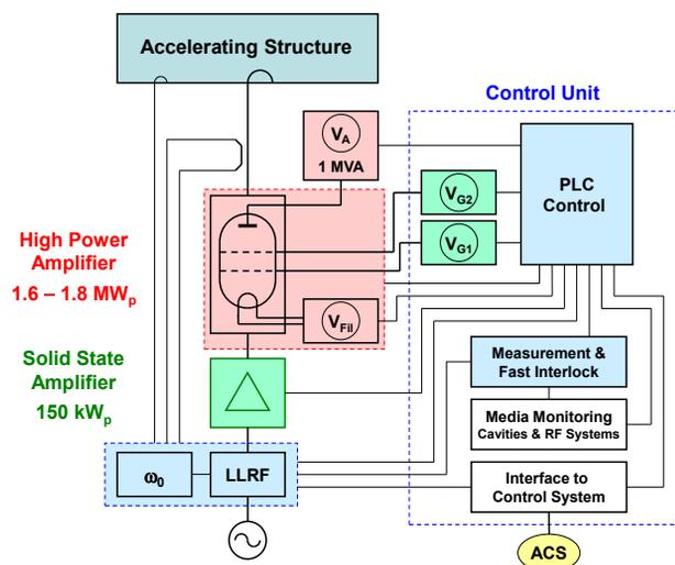
Figure 1: Simplified block diagram of the post stripper RF systems after modernisation (ACS  $\equiv$  Accelerator Control System).
