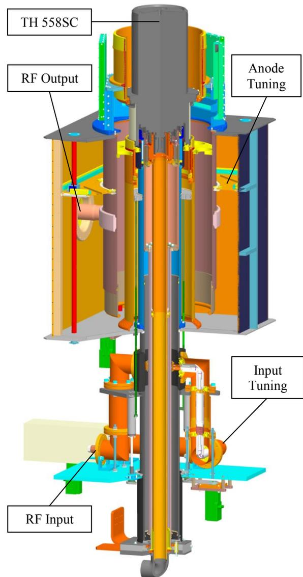
Figure 2: Sketch of the new 1.8 MW high power amplifier cavity prototype for TH 558SC designed by Thales (by courtesy of Thales Electron Devices, Thonon, France).
