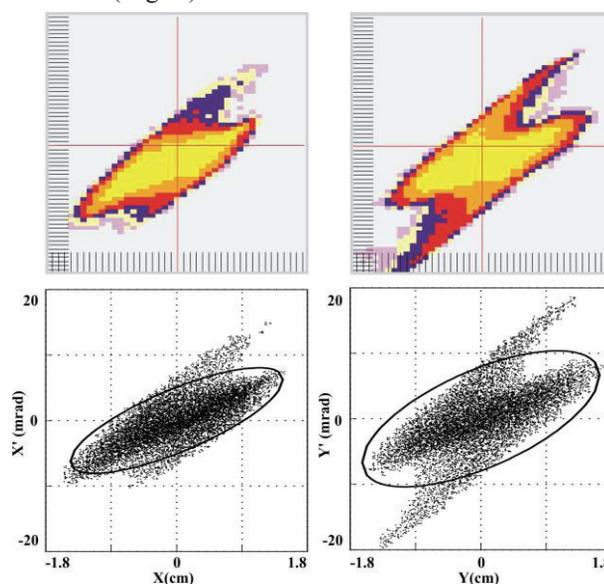
Figure 4. The measured horizontal and vertical beam emittances (top); generated macroparticles (bottom)
