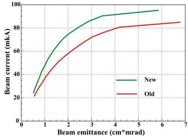
Figure 6. Beam intensity inside a given beam emittance behind HSI-RFQ with old (red) and new (green) setting for Quadrupole Quartet.
