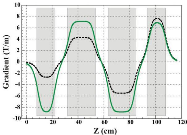
Figure 5. "Old" (dashed) and "new" (solid) magnetic field gradient along quadrupole quartet.
