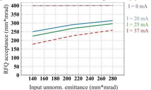
Fig. 3: "High current" acceptance of the HSI-RFQ (unnormalized) as a function of the input beam current and emittance.
