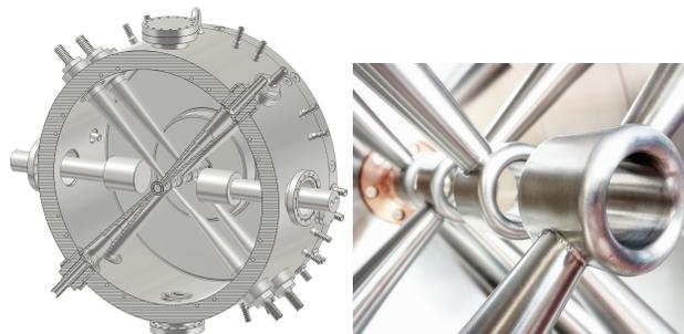
Figure 3: 3D model cross sectional view in CST MWS [6] (left) and picture of drift tubes and crossed stems (right).
