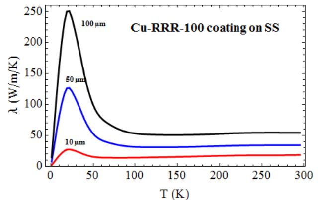
Figure 3: Thermal conductivity.
