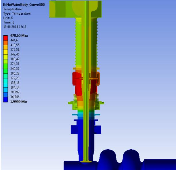
Figure 4: Thermal simulation: in case of full reflection.
