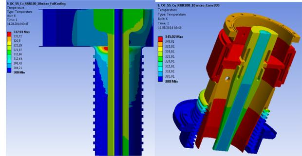
Figure 5: Thermal simulation: in case of no reflection.
