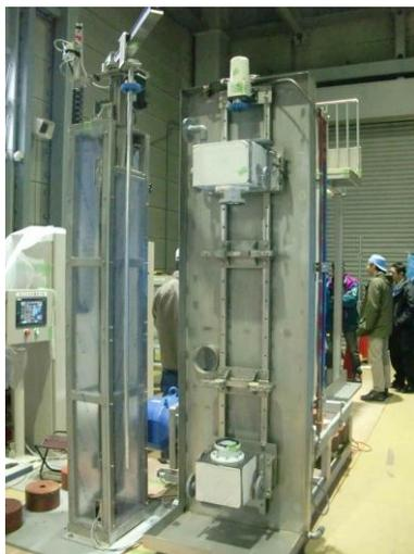
Figure 6: Cavity bed of vertical EP equipment.
