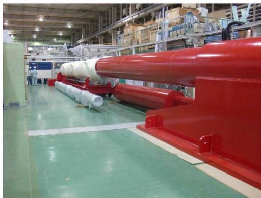
Figure 5: Picture of the ILC-type cryomodule assembly tool temporarily stored in ATF hall.
