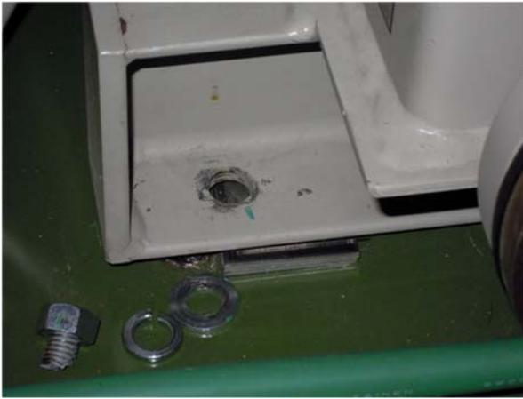
Figure 2: A broken anode-modulator anchor bolt [10].
