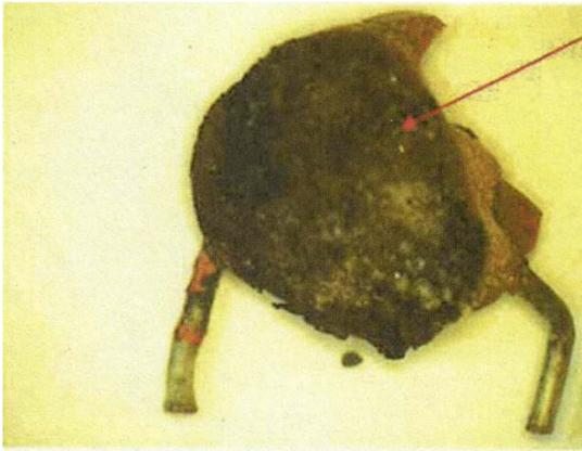
Figure 3: A carbonized ceramic condenser in the HVTR diode-stack.
