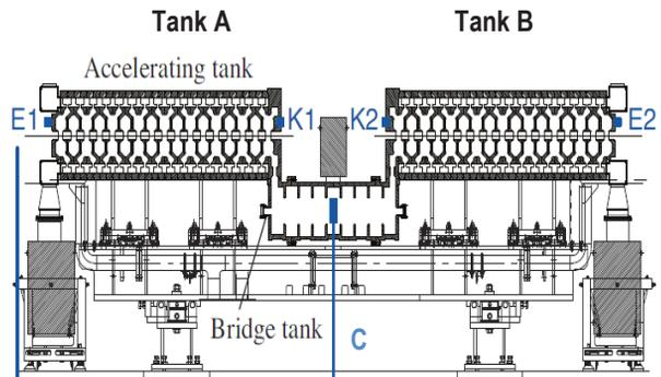
Figure 2: Sketch of J-PARC ACS cavity for acceleration.
