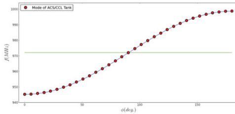
Figure 3: ACS modes shown in the Brillouin curve of the CCL cavity.
