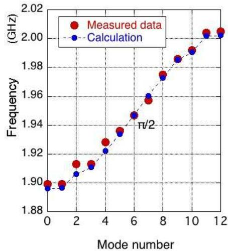
Figure 7: Dispersion curve of the ACS model cavity.
