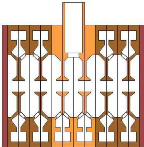
Figure 5: Cross section of the ACS model with direct RF feed.
