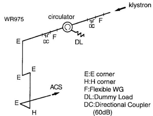
Figure 10: Waveguide system of an ACS module [4].
