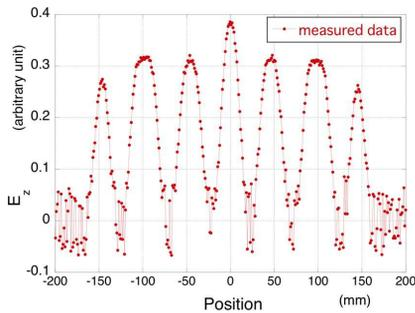
Figure 8: Measured field distribution of the ACS model.
