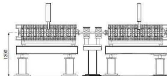
Figure 3: Schematic view of ACS without a bridge cavity.
