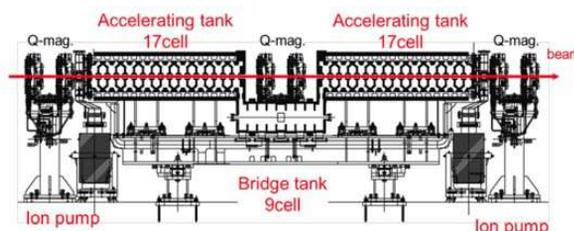
Figure 2: Cross section of an ACS module [1].
