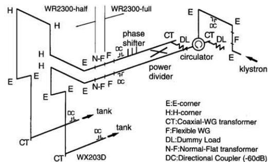
Figure 11: Waveguide system for the pair of SDTL tanks [4].
