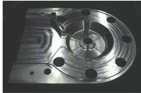
Figure 6: The center cell of the ACS model with a coupling iris.
