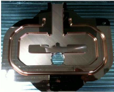
Figure 8: Halve of a power extraction coupler.
