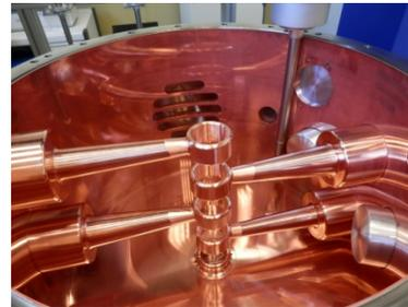
Figure 10: 5 Gap Buncher for CIEMAT.
