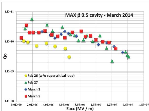
Figure 2: Measurements of the cavity performance at 2K.
