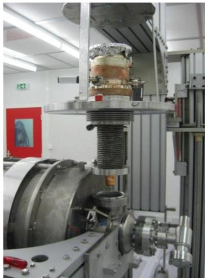
Figure 1: 5-cell SRF elliptical  $\beta=0.5$  cavity being connected to its high-power RF power coupler in clean room.
