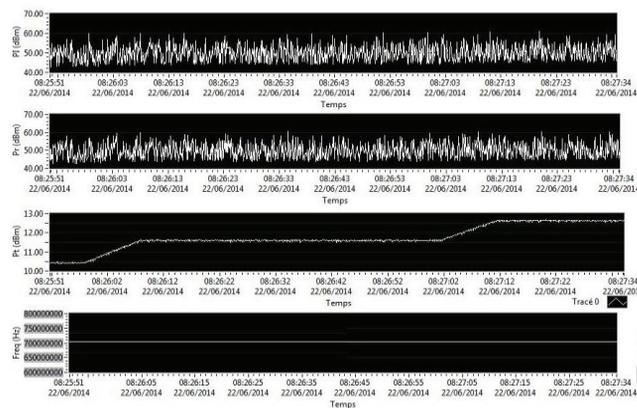
Figure 4: Measured powers during a field set-point increase.
