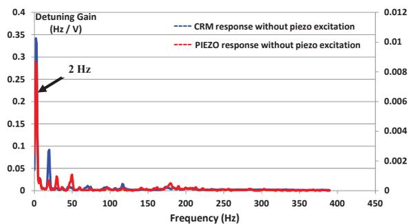
Figure 3: Measurement of microphonics background noise.
