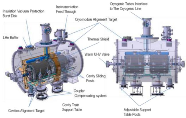
Figure 4: Cryostat
