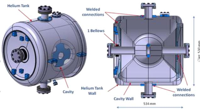
Figure 2: Cavity Mechanical Design
